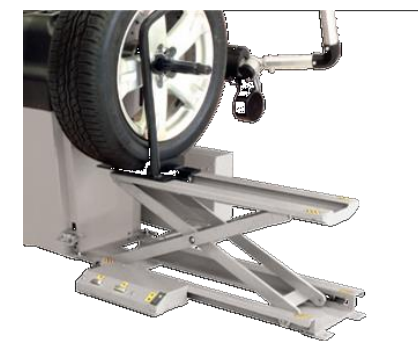
GAR324 (G-MOON) Wheel lift with Automatic compensation of wheel weight
