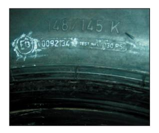
ECD = Enhanced Carcass Durability or EC : special monofilament construction (recommended mainly for mixed and off-road use).
