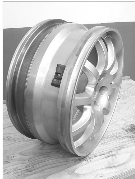
Pict. 13: PAX Wheel w/ press sensor
