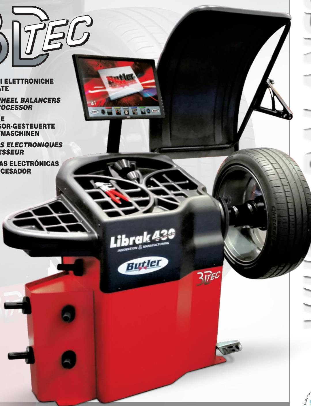
**EQUIPPED WITH AUTOMATIC WHEEL DIMENSION SONAR
